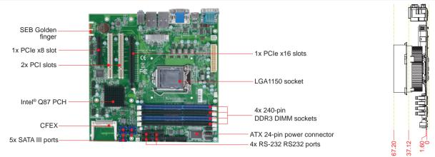
RUBY-D720VG2AR is based on Intel® Q87 chipset and desktop processor sku like Core™ i7 and i5. Build with PCI and PCI Express expensions, it is suitable for Medical, Industrial automation, and digital signage applications.
